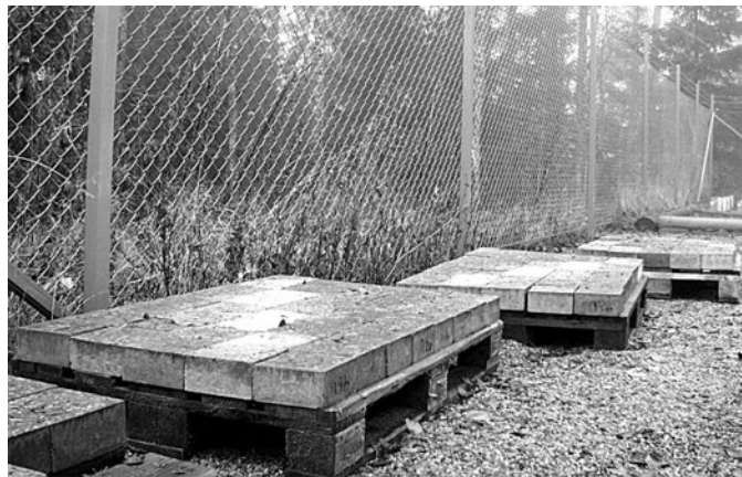
Figure 11.3 Field exposure site in an environment without salt exposure at SP's premises. Specimens are placed on pallets.
