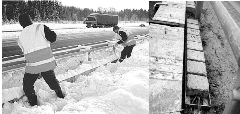
Figure 11.1 Field exposure site at Highway 40. Specimens placed in steel frames behind a guard rail (right).
