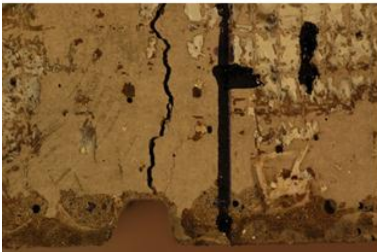
Figure 12.4: 0.2 mm crack after 28 month exposure to sea water. Concrete cover 55 mm.
