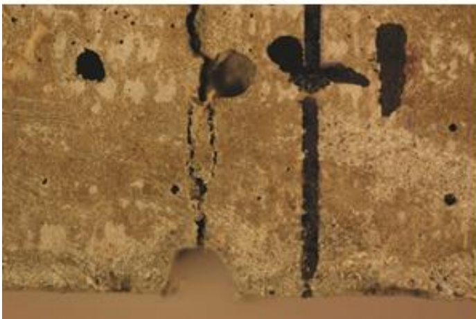
Figure 12.3: 0.4 mm crack after 28 month exposure to sea water. Concrete cover 75 mm.
