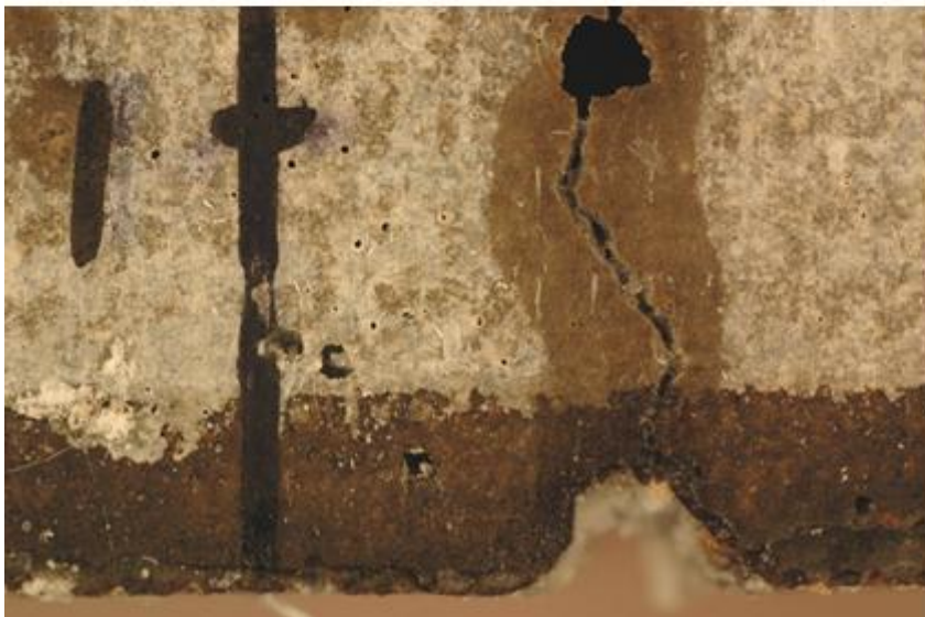
Figure 12.6: 0.4 mm crack after 28 month permanent exposure to brackish water. Upper: 75 mm cover. Lower: 55 mm cover
