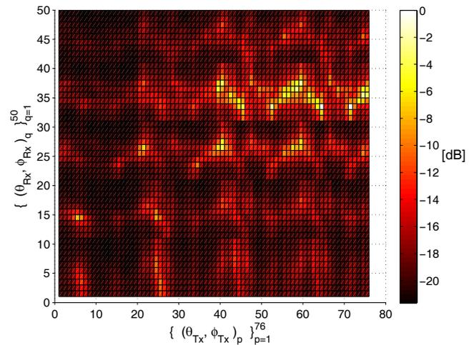
Fig. 5. Joint Capon spectrum for NLOS measurement at D1. The x-axis contains the ordered pair  $(\theta_{TX}, \phi_{TX})$  with angle ranges (in degrees):  $\theta_{TX} = [30:20:90]$  and  $\phi_{TX} = [-180:20:180]$ . The latter azimuth range is scanned per elevation angle. Similarly, the y-axis contains the ordered pair  $(\theta_{RX}, \phi_{RX})$  with angle ranges:  $\theta_{RX} = [30:20:110]$  and  $\phi_{RX} = [-90:20:90]$ .
