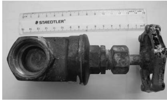
Figure A.4: In-line gate valve used in the laboratory experiments
