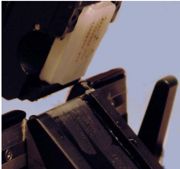
Figure 7. Sectioning of a TMA block using a microtome.
