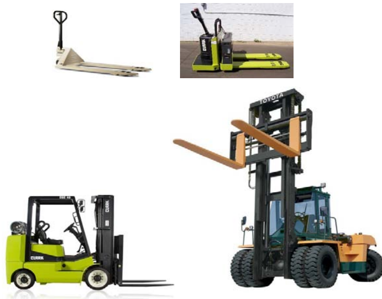
Figure 1. Different models of pallet trucks and forklifts
