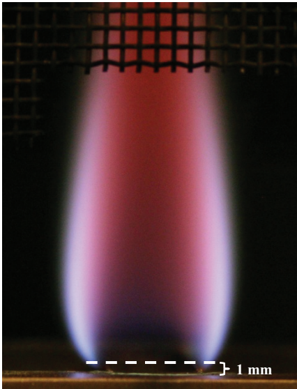
Figure 4.8. A H_2 -diffusion flame attached on a Wolfhard-Parker burner [86]. The dimension of the inner slot are 40\text{ mm} \times 8\text{ mm} and of the two outer slots 40\text{ mm} \times 16\text{ mm} (length \times width), respectively.
