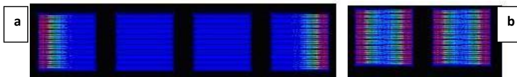
Figure 5.1.2: Schematic representation of samples (Build-III) with different scan length, a) ~ 50mm b) 10mm
