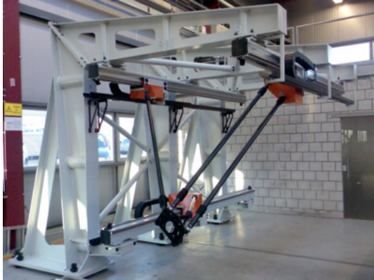
Figure 1.1 Gantry-Tau prototype developed within the SMErobot project.
