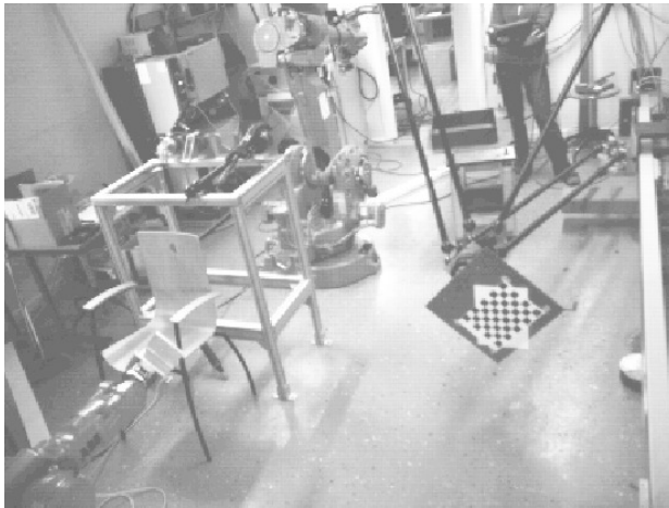
Figure 5.25 View out of the camera: The robot with the calibration pattern (to the right in the picture). To the left in the picture, obstacles, e.g., experiment equipment and and ABB IRB 2400 robot can be seen.
