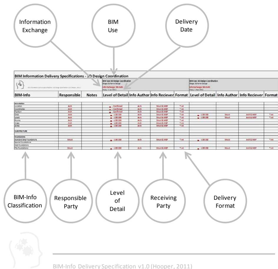
Figure 11: BIM-Info Delivery Specification – Constituent Parts
