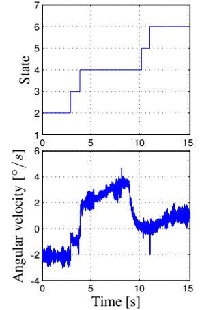
Fig. 7. Measured angular velocity in the redundant direction.
