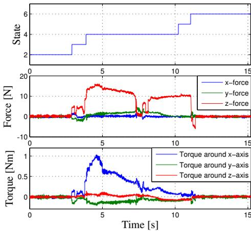
Fig. 5. Force data from an assembly sequence vs. time. The uppermost diagram shows the state sequence, the middle the forces (along the first three feature coordinate directions, i.e. they are given in frame  $f1$ ) and the lowermost the torques (around the coordinate axes defined by the quaternion, i.e., they are given in frame  $f2$ ).
