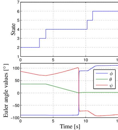
Fig. 6. Calculated Euler angles from the assembly sequence.  $\phi$  is the first rotation around the  $z$ -axis,  $\theta$  the rotation around the  $y$ -axis, and  $\psi$  the final rotation around the  $z$ -axis. Problems occur when the singular position is entered just before  $t = 9$  [s].
