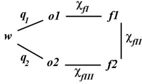
Fig. 2. The inverse kinematics problem is solved by considering the position loop constraint that is defined by the kinematic chain,  $w$  denoting the world coordinate frame,  $q_1$  and  $q_2$  robot joint coordinates,  $o1$  and  $o2$  object frames,  $f1$  and  $f2$  feature frames, and  $\chi_f = (\chi_{fI}, \chi_{fII}, \chi_{fIII})$  the feature coordinates.
