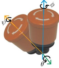
Fig. 4. Illustration of the Euler angle representation (ZYZ) of the orientation of the button.  $\phi$  is a rotation around the  $z$ -axis,  $\theta$  is then a rotation around the  $y$ -axis in the new coordinate system defined by the first rotation. Finally  $\psi$  is a rotation around the new  $z$ -axis.
