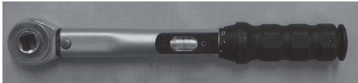
Figure 5. The adjustable spanner, used to apply different torques (Nm) during the measurements of knee rotation.
