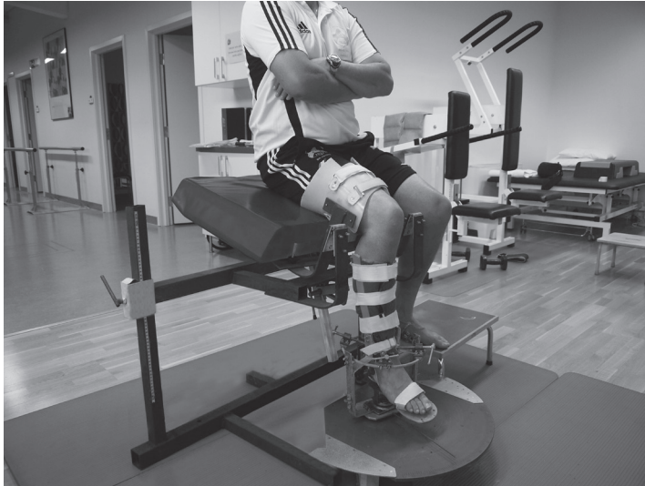
Figure 2. The Rottometer with a test person fixed to the device ready to be measured at 60° of knee flexion angle.
