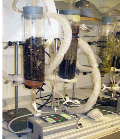
Figure 4. (a) A single-stage leach bed reactor for methane production, and (b) the UASB reactor used in the two-stage system. The photograph shows two-stage anaerobic digestion of mussels (left) and reeds (right).
