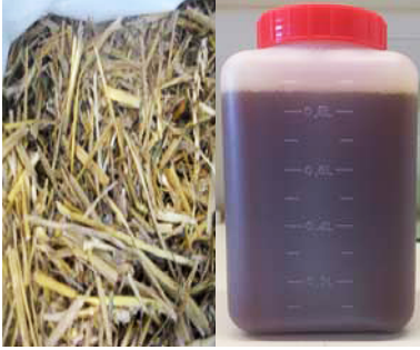
Figure 9. The original wheat straw and the sugar-rich liquid obtained after steam and enzyme pretreatment.
