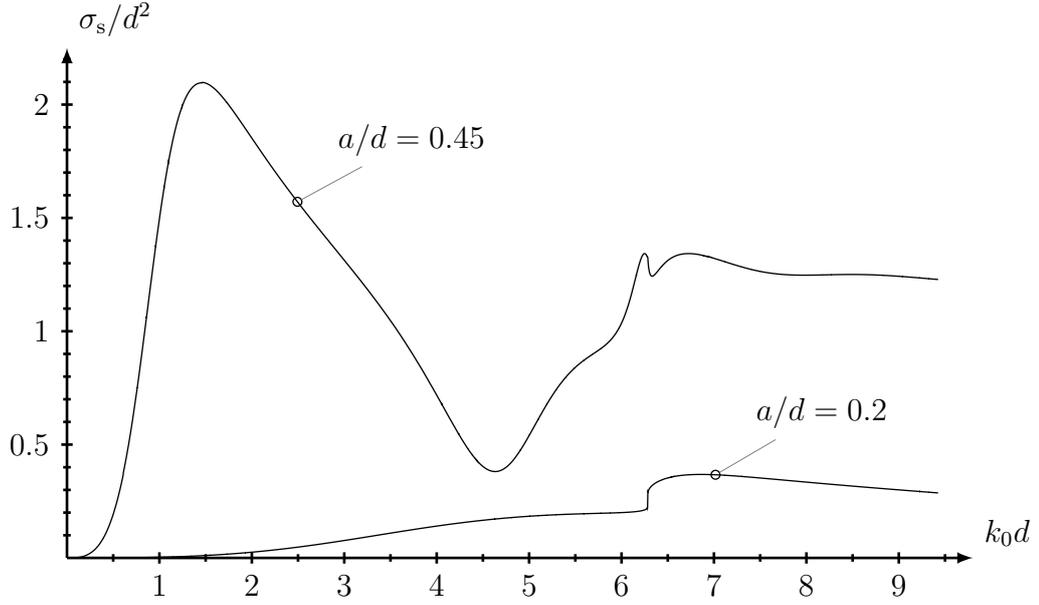
**Figure 9:** The scattering cross section,  $\sigma_s$ , for a PEC sphere of radius  $a$ , centered at the origin, as a function of  $k_0d$  and vertically polarized incident plane wave. The cross section is scaled with  $d^2$ . The locations of the planes are  $z_+/d = 0.5$  and  $z_-/d = -0.5$ .
