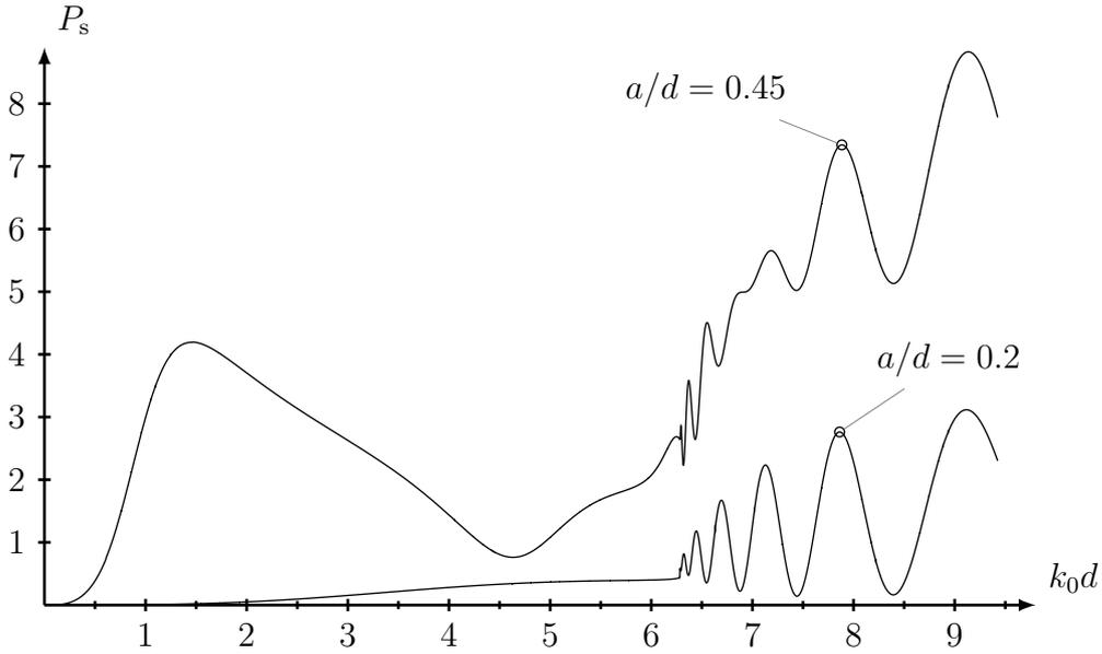
**Figure 8:** The scattered power  $P_s$  by a perfectly conducting sphere, centered at the origin, as a function of frequency,  $k_0 d$ , for a vertical electrical dipole, see (11.1), located at  $\mathbf{r}_0 = -x_0 \hat{\mathbf{x}} + z_0 \hat{\mathbf{z}}$ , where  $x_0/d = 10$  and  $z_0/d = 0$ . The locations of the planes are  $z_+/d = 0.5$  and  $z_-/d = -0.5$ .
