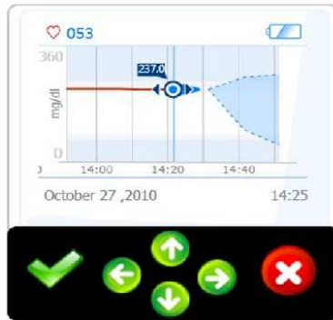
Figure 2.3 User Interface of the DIAdvisor system patient application implemented on the UMPC. On the screen, the user can follow the present and recent glucose values together with a projected future trajectory within specified uncertainty limits. Other vital signs, such as heart rate (see upper left screen corner), may also be possible to follow. User inputs, regarding, e.g., insulin and meal intake, are provided by a menu system controlled by the buttons at the bottom of the screen. Reproduced from [The DIAdvisor Consortium, 2012].
