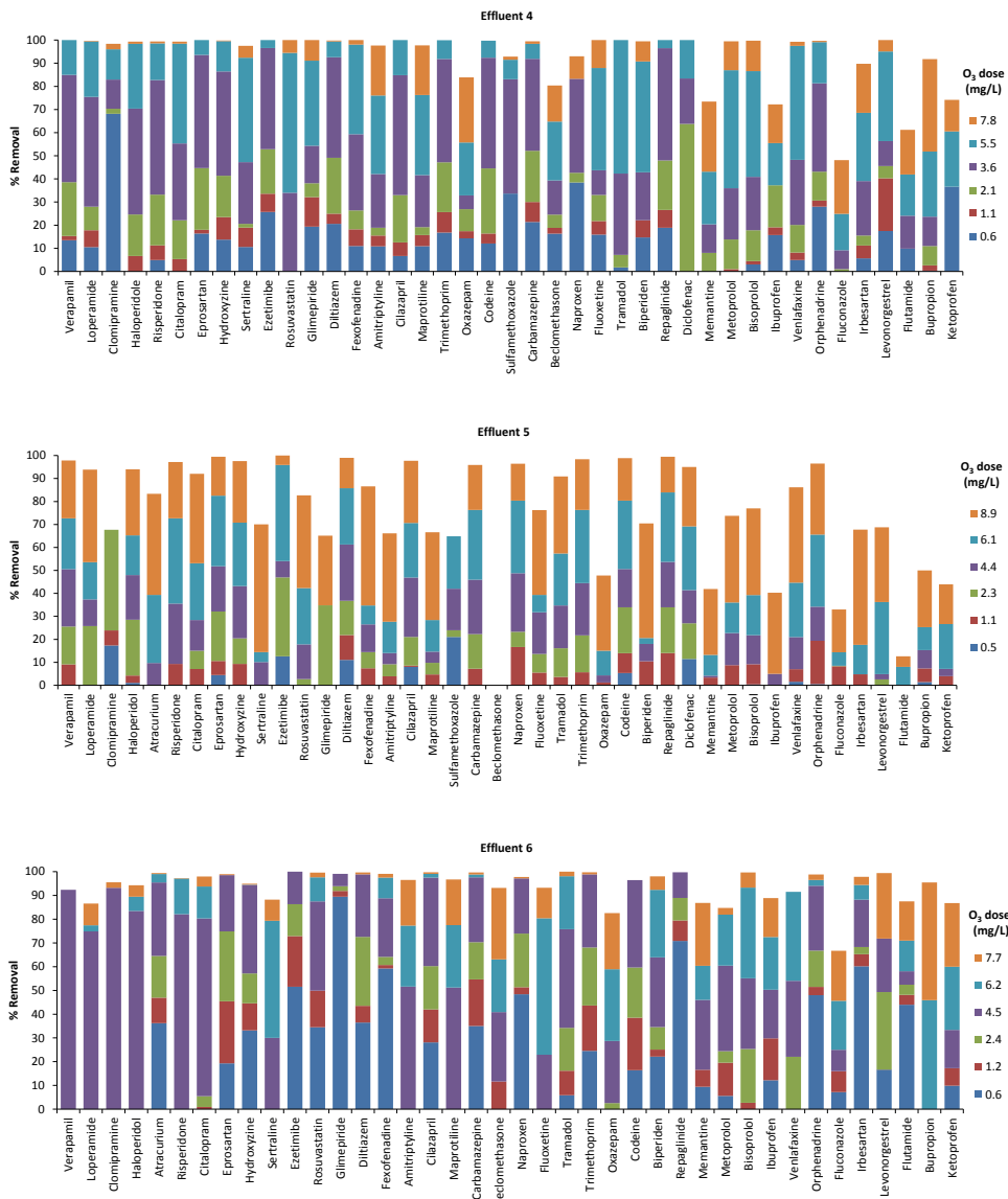
Figure S1: Profiles of dose dependency for the removal of pharmaceuticals in the 6 investigated wastewaters.
