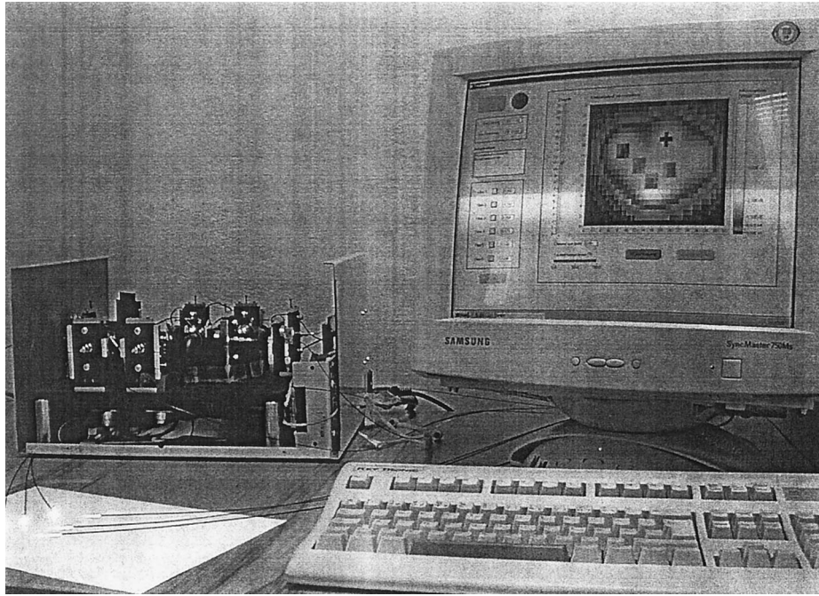
Fig. 3. Photograph of the system with six emitting fibers and a dosimetry chart displayed on the computer screen.
