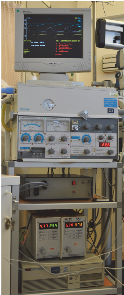
Fig. 2. Experimental set-up used in paper II, III and IV. From top to bottom: Computerscreen, ServoVentilator 900C, A/D converter, CO2 analysers and computer.
