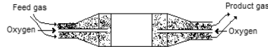
Fig. 1: Reactor setup with two heat buffers, each with its own oxygen inlet.
