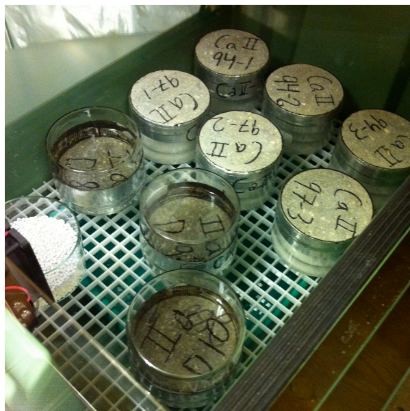
Fig. 13 One of the climate boxes with a glass lid containing nine cups, three of which inverted. The fan is visible to the left and the CO 2 -absorbent beneath it.
