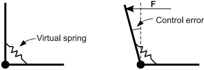
Figure 10.1 Illustration of how the joint torques are estimated. The controlled joint acts as a virtual spring, and when a force is applied to it, the deflection is used to estimate the joint torque.
