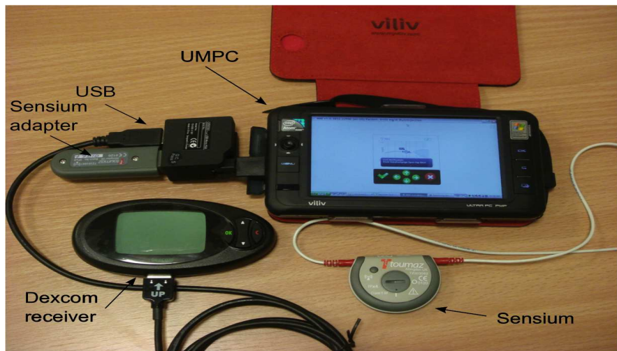
Figure 3.5 DIAdvisor I and II trials equipment. The ultra mobile PC ( center ) is connected via USB to the Seven®Plus receiver ( left ) and the Sensium™ Life Pebble ( bottom ) through its dedicated adapter.
