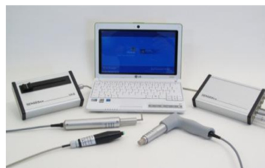
Fig 5b. Quantitative Sensory Test equipment (Somedic AB, Hörby Sweden); computer, sensbox, electronic algometer, electronic von Frey transducer, VAS response unit and hand held switch. The VAS response unit was not used in this study.
