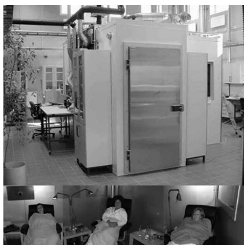
FIG. 1. (above) The stainless steel chamber at the University of Lund. (below) The arrangement of test subjects (in this case female volunteers) inside the chamber.
