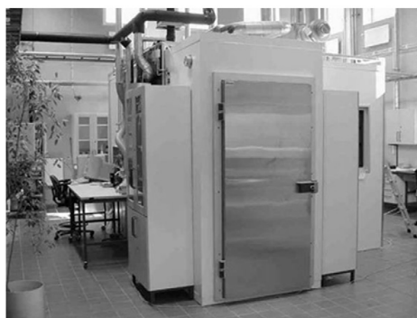
Fig. 1. The stainless steel exposure chamber at Lund University.
