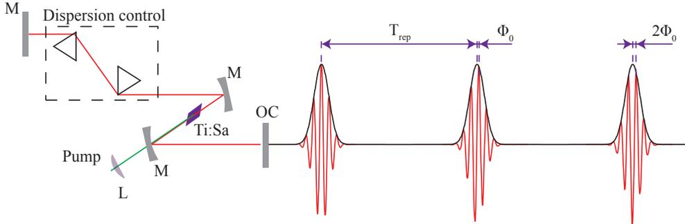
**Figure 2.6:** Typical geometry of a femtosecond resonator cavity; M - mirror, OC - output coupler, L - pump focusing lens.
