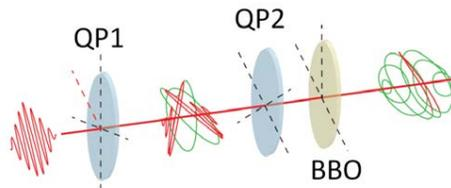
Figure 3: Double optical gating setup, from ref.<sup>9</sup>. QP1 and QP2 - quartz plates, BBO – barium borate crystal.
