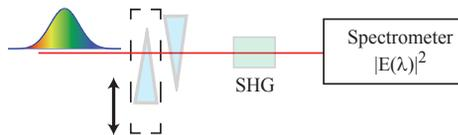
**Figure 2.8:** Sketch of the d-scan experimental setup.
