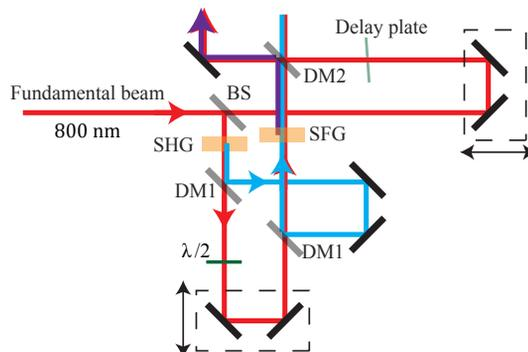
**Figure 4.18:** Two-color  $\omega/3\omega$  interferometer; BS - 50:50 beam splitter for 800 nm, DM1 - dichroic mirror with HR@ 400 nm and HT@ 800 nm, DM2 - dichroic mirror with HR@ 267 nm and HT@ 800 nm, SHG - KDP crystal for Type I second harmonic generation, SFG - KDP crystal for Type I sum frequency generation,  $\lambda/2$  - half wave plate for 800 nm.
