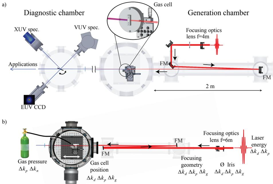
**Figure 4.13:** a) HHG setup configured for 4 m focusing with a lens; b) Setup parameters controlled for phase-matching optimization. The setup is that corresponding to a 6 m focus. FM - folding mirror.
