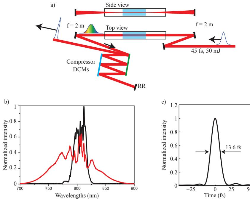
**Figure 3.6:** a) Post-compression setup, RR - retro reflector, DCM - double chirped mirrors; b) Pulse spectrum before (black line) and after (red line) post-compression; c) Pulse duration after post-compression.
