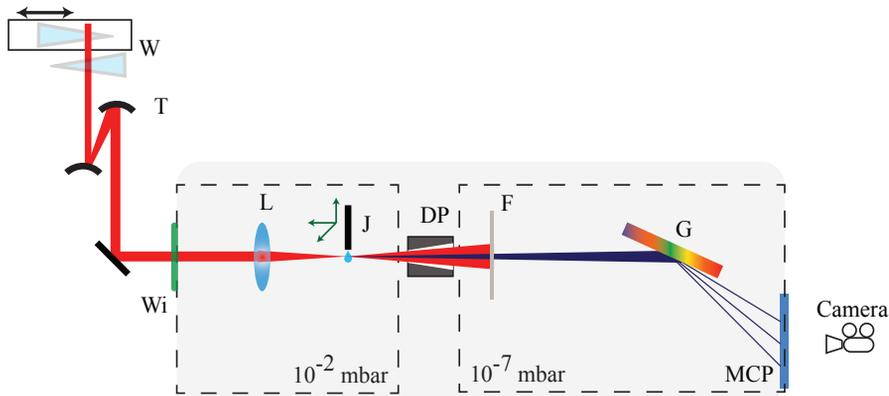
**Figure 4.14:** The HHG setup; W - wedge, T - reflective telescope,  $W_i$  - vacuum entrance window, L - achromatic lens, J - argon gas jet, DP - differential pumping hole, F - motorized filter mount, G - diffraction grating, MCP - microchannel plate with phosphor screen.
