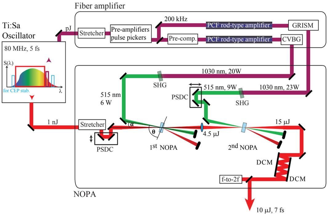
**Figure 3.11:** The OPCPA system; PCF - photonic crystal fiber, CVBG - chirped volume Bragg grating, SHG - second harmonic generation in BBO crystals, PSDC - pump-signal delay control, NOPA - non-collinear optical parametric amplification in BBO crystals,  $\alpha$  - non-collinear angle,  $\theta$  - phase-matching angle, DCM - double chirped mirror.
