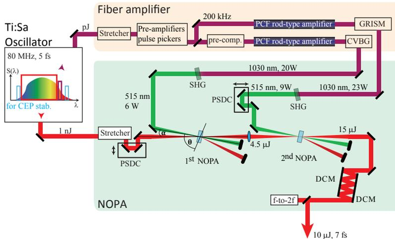
**Figure 1.** The OPCPA system; PCF - photonic crystal fiber, CVBG - chirp volume Bragg grating, SHG - second harmonic generation in BBO crystals, PSDC - pump-signal delay control, NOPA non-collinear optical parametric amplification in BBO crystals,  $\alpha$  - non-collinear angle,  $\theta$  - phase-matching angle, DCM - double chirp mirror.
