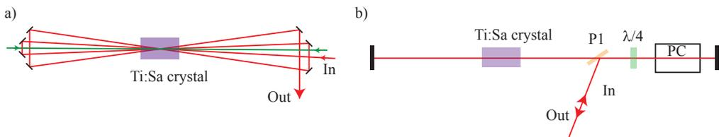
**Figure 3.3:** a) Multi-pass and b) regenerative amplifiers.
