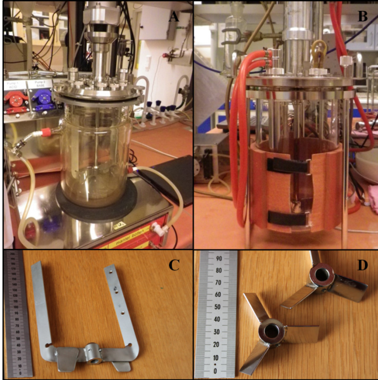
Figure 3.6. Experimental set-up. The more advanced hydrolysis reactor Hanna (A) and the standard bioreactor, Biostat A+ (B). The Hanna system was equipped with an anchor impeller (C) and the Biostat reactor with a pitched blade impeller (D).
