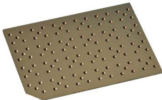
Figure 16. A photograph of an ISET chip produced in silicon.
