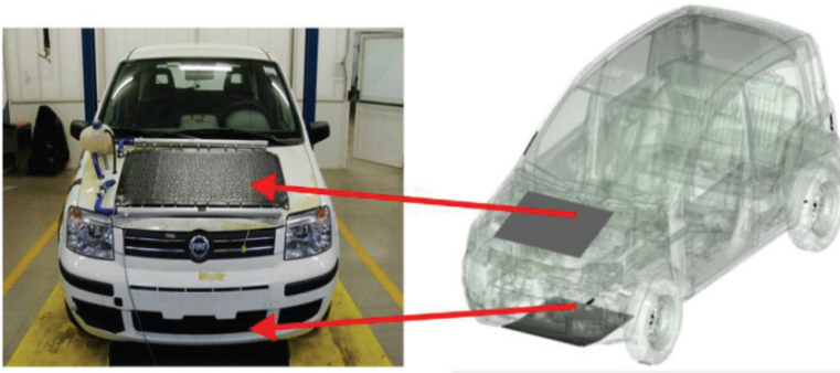
Fig. 2.3 Different positions of HEXs in a vehicle [18].
