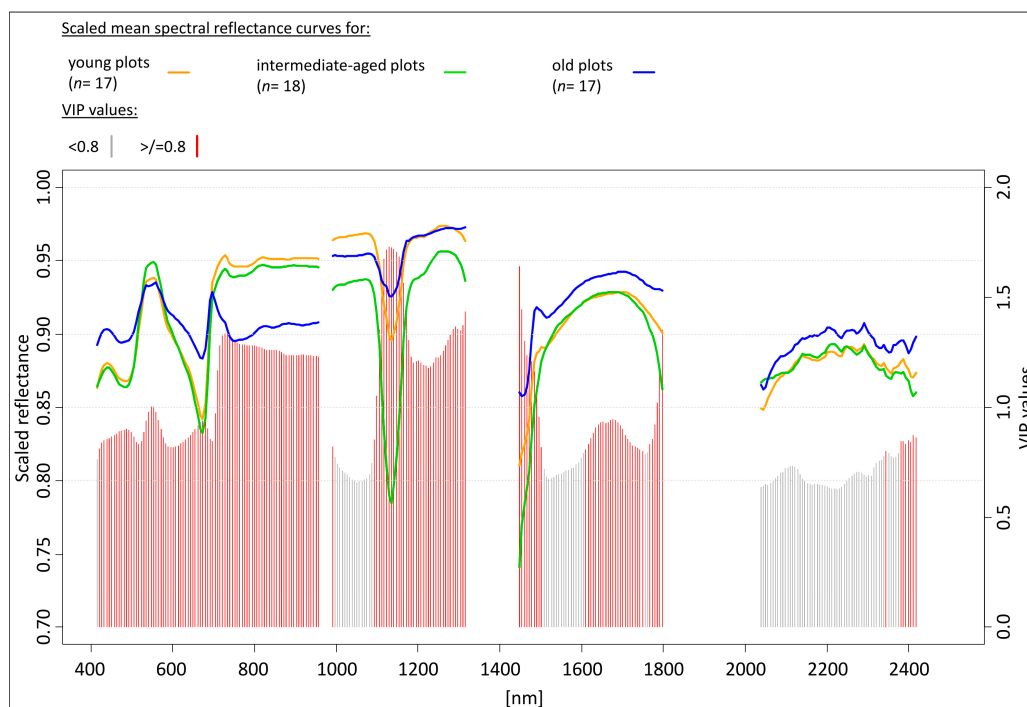
Figure 4. VIP values as a function of the wavelengths used in Model 1 (the PLS-DA model developed from the full set of HySpex hyperspectral wavebands) ( n = 269 ). The higher the VIP value of a waveband, the greater its contribution to the model. The most influential wavebands in the PLS-DA model (with VIP values >0.8 ) are marked in red. The orange, green, and blue lines represent the scaled mean spectral reflectance curves obtained using the training subsets for young, intermediate-aged, and old grassland plots, respectively.
