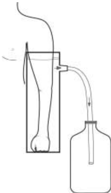
Figure 4. The arm volume was measured with the water displacement method (Archimedes principle). The arm was submerged in a container with water and the displaced volume was weighed.
