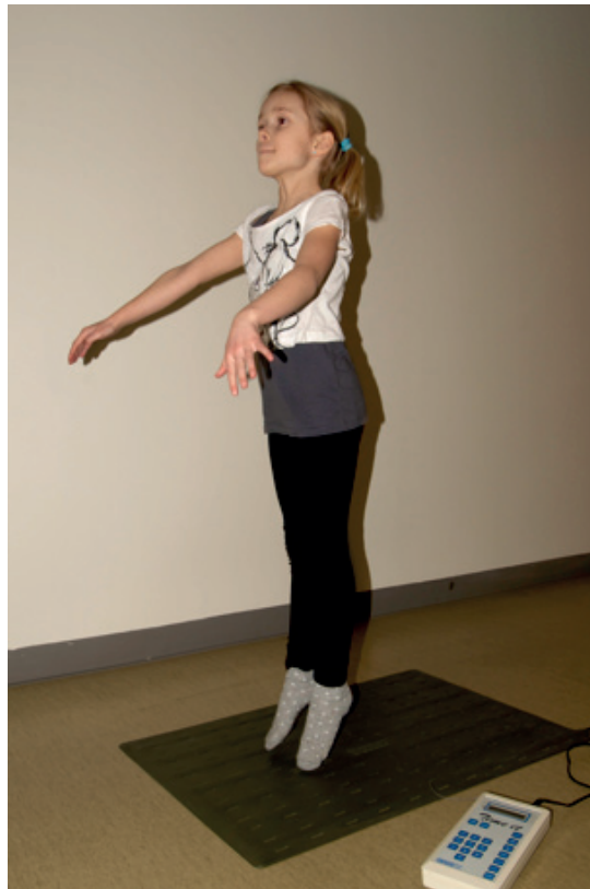
Fig 18. VJH performed on the “Time it” electronic mat. By courtesy of Bjarne Löfgren
