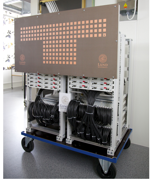
Fig. 3. Left: Side view of the mechanical assembly of the BS. The two racks sit side-by-side (not as shown) with the SDRs facing the same direction (towards the antenna array). Two columns of URSPs are mounted in each rack, totaling 50 of them. Right: Picture of the assembled BS, with mounted antenna array.
