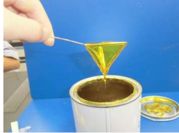
Figure 5. We pulled up the frame out of the resin liquid
