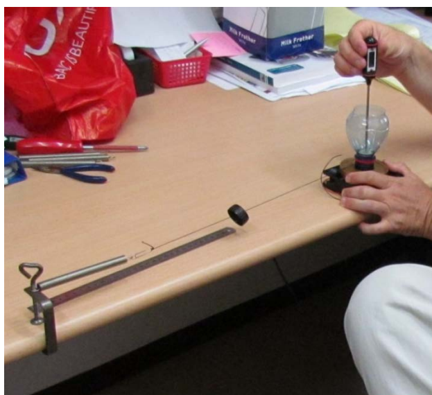
Figure 4: Measuring energy change via the rise in temperature in a spring contraction process
