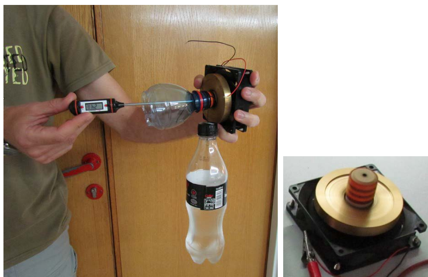
Figure 1. The desktop Joule device. The operating fully assembled device (left) and the spinning part (right)
