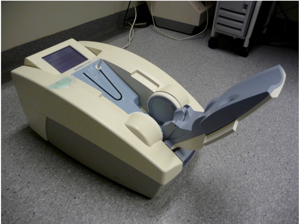
Figure. 17 A quantitative ultrasound apparatus
