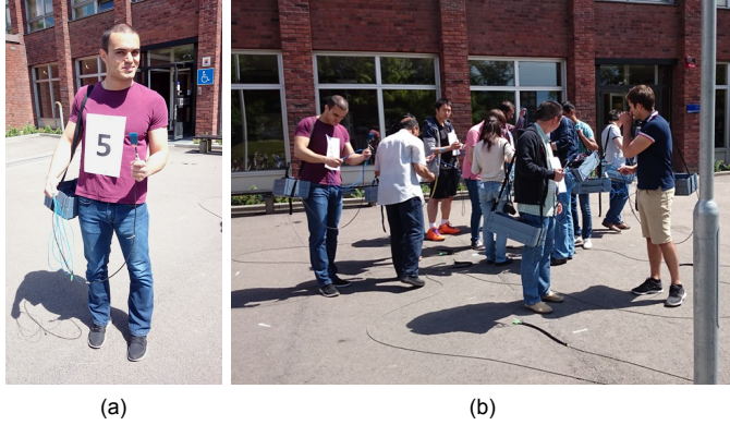
Fig. 2. (a) A user holding the user equipment antenna with an inclination of 45^\circ . (b) Users moving randomly within the five-meter diameter circle.
