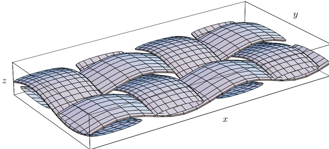
**Figure 1:** The geometry of the glass fiber.
