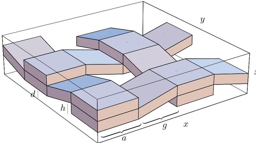
**Figure 6:** A simple model of a woven composite material.
