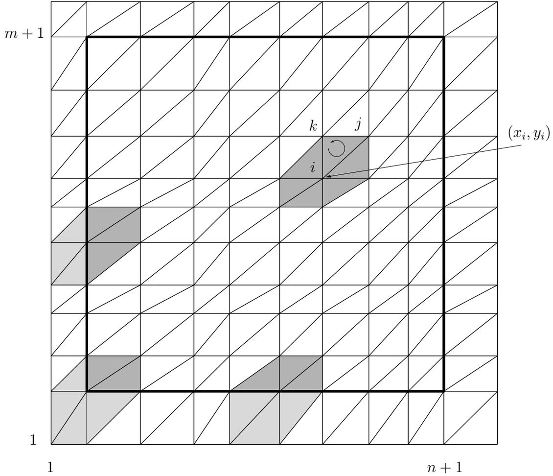
**Figure 2:** The mesh of the extended unit cell, the unit cell (heavy line), and the support of the functions  $\lambda_i(x, y)$  centered at an interior point, at two edge points, and at a corner point of the unit cell. Areas with lighter shading represent the support of the function  $\lambda_i(x, y)$  outside the unit cell.
