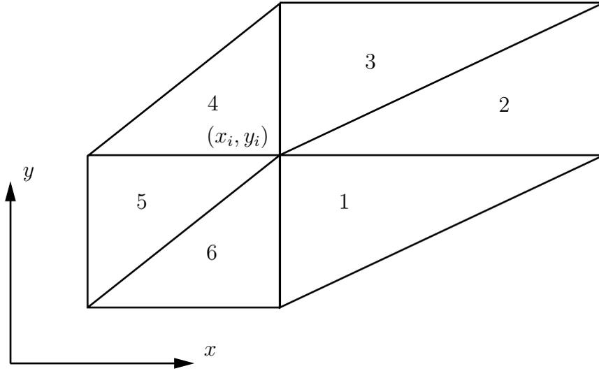
**Figure 10:** The support of the function  $\lambda_i(x, y)$  and the different areas of the support of the functions  $\phi_i^p(x, y)$ ,  $p = 1, 2, 3, 4, 5, 6$ .
