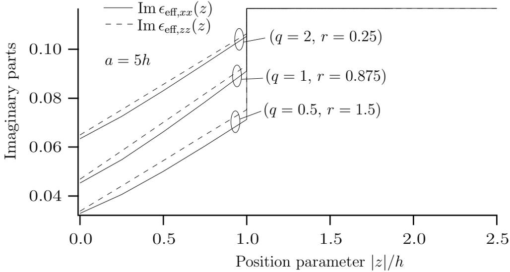
**Figure 8:** Imaginary parts of the effective permittivity components of three different weaves.
