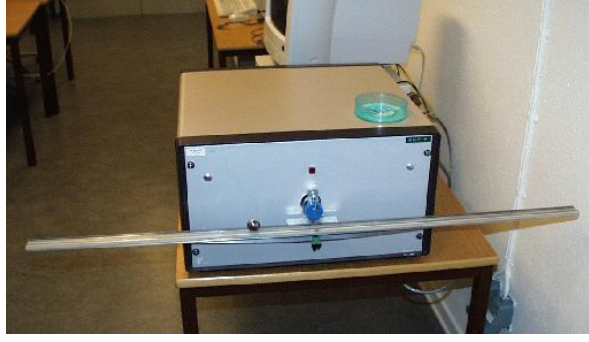
Figure 2 The ball-and-beam laboratory process.
