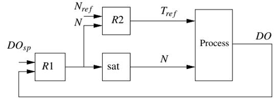
**Fig. 5** A block-diagram over the mid-ranging controller. Sat stands for saturation. R1 is used even when 'only'  $N$  is controlling the dissolved oxygen, a gain scheduled PID. R2 is a PID controller.
