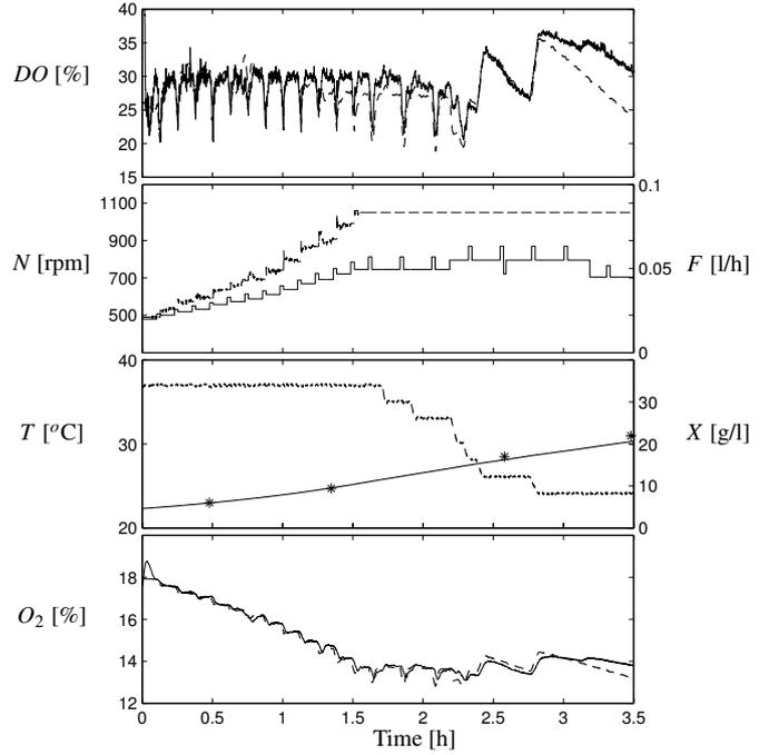
**Fig. 3** Simulation of the model together with experimental data. From top: dissolved oxygen  $DO$  (simulation dashed), stirrer speed (dashed)  $N$  and feed  $F$ , temperature  $T$  (dashed) and cell mass  $X$  (experimental data '\*'), oxygen concentration in the outlet gas  $O_2$  (simulation dashed). Time [h] after feed-start.
