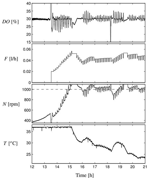
**Fig. 6** Experiment using the modified probing strategy together with the temperature limited fed-batch technique. The fed-batch part of the cultivation is shown. From top:  $DO$  dissolved oxygen,  $F$  feed,  $N$  stirrer speed,  $T$  temperature.  $N_{ref}$  is dashed. At  $t = 18.2$  h antifoam is added which has a large impact on the dissolved oxygen signal.
