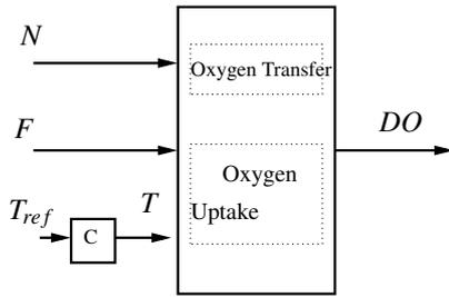
**Fig. 4** A description of the process. Stirrer speed,  $N$ , Feed,  $F$ , Temperature  $T$ , Temperature reference  $T_{ref}$ , dissolved oxygen  $DO$  and a temperature controller  $C$ .  $C$  is typically a pulse width modulation of the cold and hot water flows.
