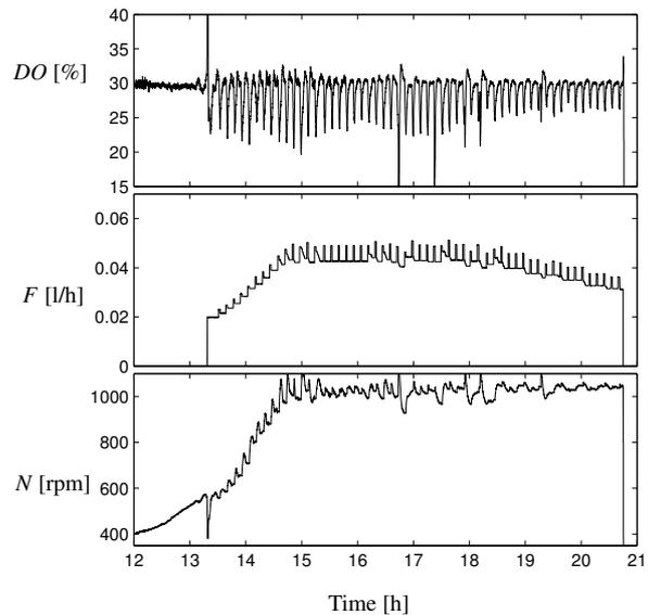
**Fig. 2** A cultivation where the original probing feeding strategy is used. The fed-batch part of the cultivation is shown. From top: dissolved oxygen  $DO$ , Feed  $F$  and the stirrer speed  $N$ . At  $t = 16.7$  h and  $t = 17.5$  h antifoam is added which has a large impact on the dissolved oxygen.
