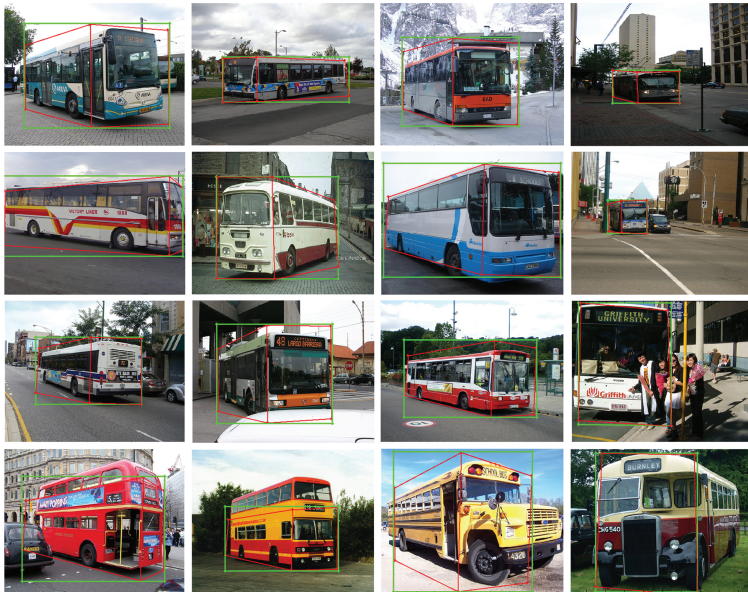
Figure 8.8: Example results. Detected bounding boxes are shown in green and their layout in red. The first three rows shows correctly detected objects with roughly correct pose. The method was able to automatically handle cases when only one side is visible. The last row shows the buses of which the pose estimation is less accurate.
