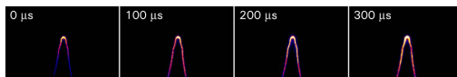
FIG. 3. (Color online) Time-resolved images of PLIF of formaldehyde in a laminar premixed flame.
