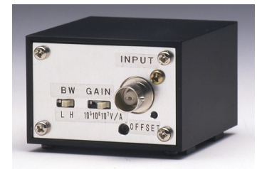
Figure 5.8. Typical view of a standardized transimpedance amplifier (C7319, Hamamatsu).
