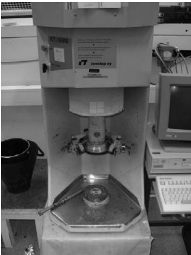
Figure 6.1. The ICT-150 RB gyratory compactor at VTI, Linköping.
