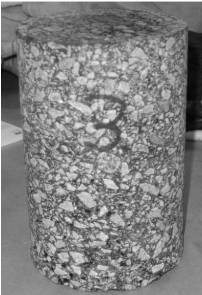
Figure 6.3. A cored and cut uniaxial specimen.
