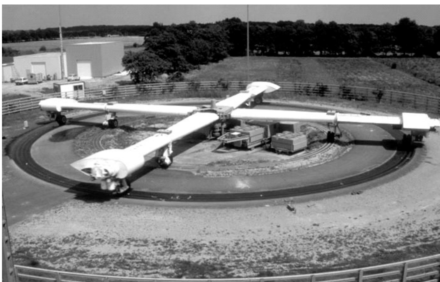
Figure 3.31. The LCPC circular test track (TRB Committee on FS/APT, 2006).
