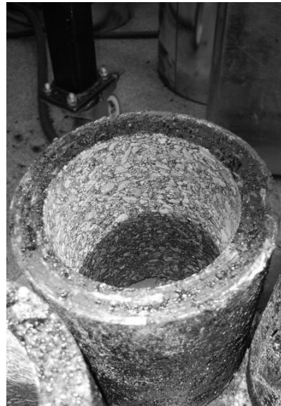
Figure 6.4. The outer shell of the gyratory compacted plug.
