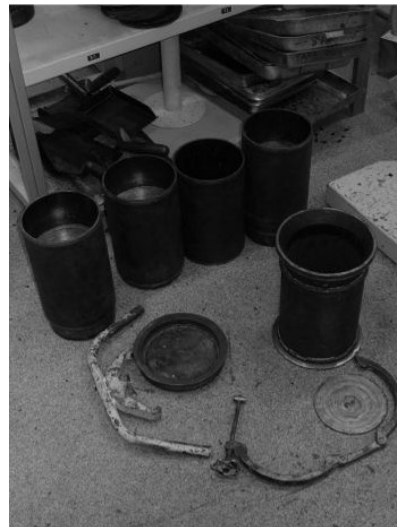
Figure 6.2. The mould and its components.
