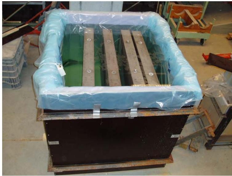
Figure 2: Concrete slabs submerged in saline water in the laboratory
