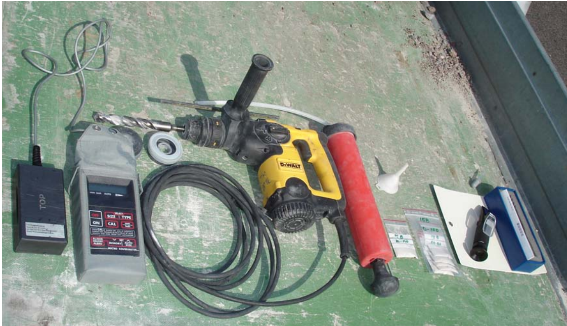
Figure 11: The equipment used when sampling dust by dry drilling in the ports of Malmö and Trelleborg
