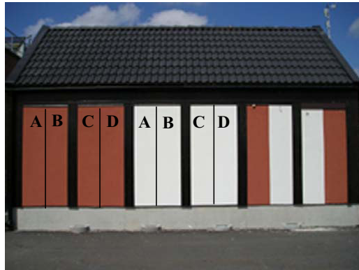
Figure 5.25 Test house with four new façade elements (the south-facing side is shown); A: mineral rendering with addition of biocides; B: mineral rendering without addition of fungicides; C: organic rendering with addition of fungicides; D: organic rendering without addition of biocides
