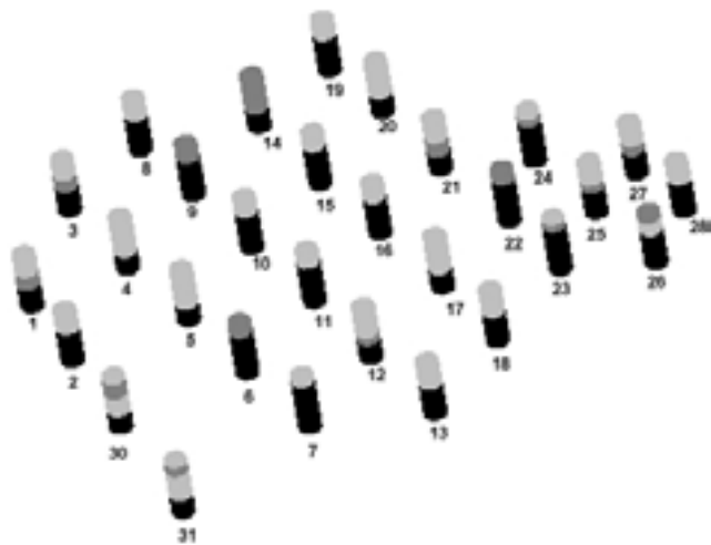
Fig. 3: Result of auger drilling investigation, view from SW. Legend: dark grey, clay; black, waste; light grey, other materials, often mixed (sand, gravel, clay till, lime, mould, sludge, bricks). Vertical enlargement: \times 10 .
