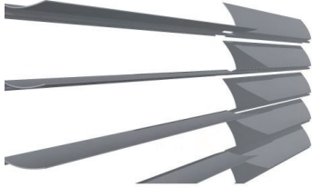
Figure 2: Illustration of the reflectors from the interior with one section in an opened mode (left) and one in a closed mode (right).
