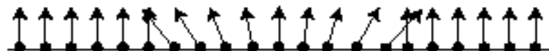
Fig.16. Cross-section of a similar bump with haptic bump mapping. This can be done with a 2D haptic device.
