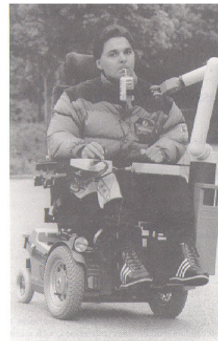
Picture No. 11. A user drinking with the help of the Manus arm.
