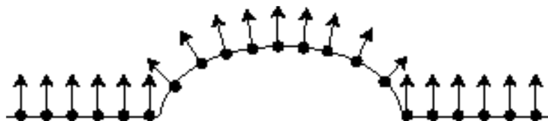
Fig. 15. Cross-section of a bump on a plane with interaction point positions and forces using real 3D haptics.
