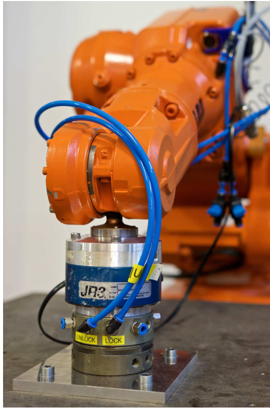
Figure 6.3 Experimental setup for joint identification, comprising an ABB IRB140 6-DoF robot manipulator. The end-effector is rigidly attached to the table during the measurement procedure, thus locking all the DoF of the robot.
